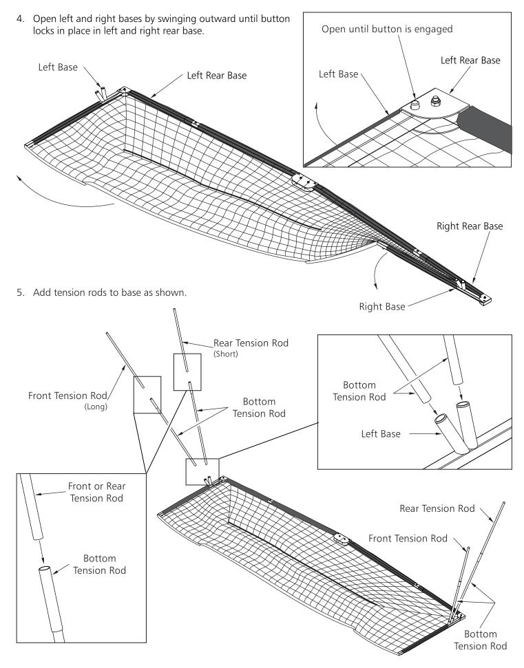
6. Connect top corners of net to front tension rod assembly by sliding rod cap over end of tension rod.
